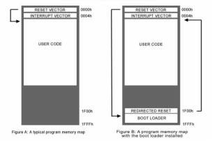
The diagram above shows the memory map of a program with and without the bootloader installed.
